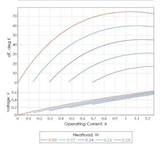
**Note**: Performance data is specified for optimal conditions (TEC hot side is stabilized at ambient temperature). Heatsink thermal resistance is not included into estimations. Use TECCad Software for estimations under different conditions.
